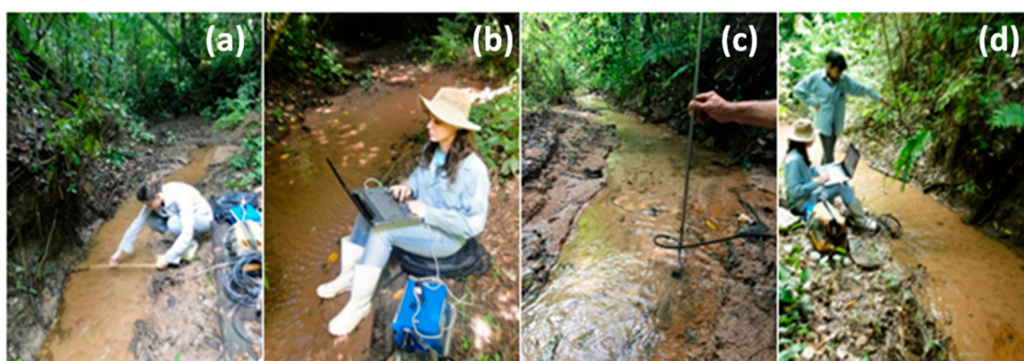
Figure 6. Flow data collection with the portable ISCO 2150 m: (a) width section measurement ( \text{cm} ) of a watercourse; (b) input parameters; (c) sensor in a watercourse; (d) reading flow and data storage.
